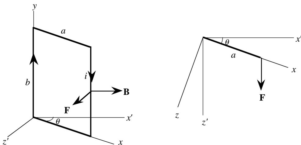
The right diagram shows the view from above. The magnitude of the torque is given by
