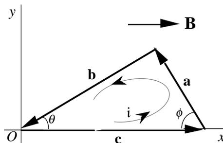
(b) The sum of forces on the three sides is  $\mathbf{F}_a + \mathbf{F}_b + \mathbf{F}_c = (-iaB \sin \phi)\mathbf{k} + (ibB \sin \theta)\mathbf{k} = 0$ , where we noted that  $a \sin \phi = b \sin \theta = ab/c$ . This is in fact a special case of 50P, part (b).
