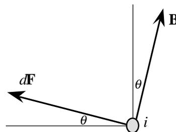
Now sum the forces on all the segments of the loop. The horizontal component of the total force vanishes since each segment of wire can be paired with another, diametrically opposite, segment. The horizontal components of these forces are both toward the center of the loop and thus in opposite directions. The vertical component of the total force is
