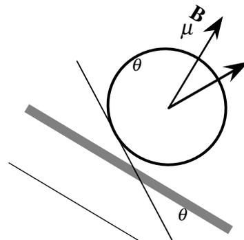
rectangular with two sides of length  $L$  and two of length  $2r$ , so its area is  $A = 2rL$  and the dipole moment is  $\mu = NiA = 2NirL$ . Thus  $mgr = 2NirLB$  and
